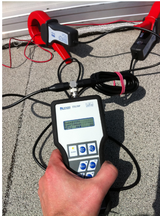
Illustration 07: Application of Ground-fault location kit
